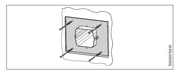
► Secure the base plate to the wall with four screws.
