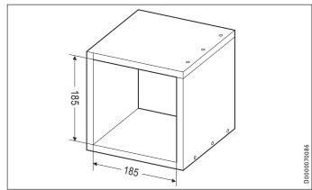
For a cavity wall, construct enclosed wooden edging with a length corresponding to the wall thickness between the internal lining and external cladding.
