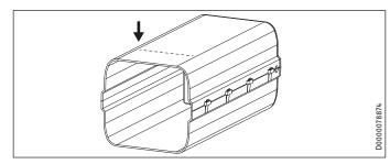
► Shorten the wall mount casing so that it protrudes over the external panel base plate by the length illustrated.
