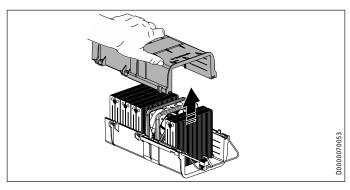
Lift off the top half of the fan unit.
