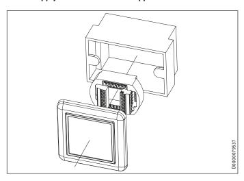
The control unit and the programming unit are installed in a flush box. The power supply unit is installed on a top-hat rail in the fuse box. The power supply unit requires up to 4 MCB spaces.
