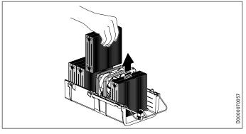
► Remove the heat exchange sections.
