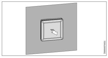
Carefully pull the internal panel cover slightly back from the wall.
