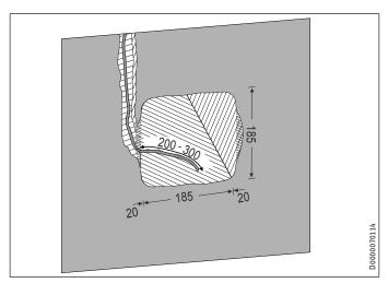
► Create a wall outlet vertical to the wall without a fall.
