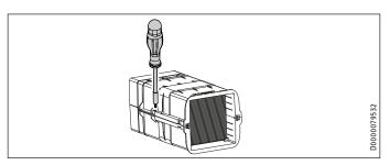
▶ Undo the screws on the long sides of the fan unit.
