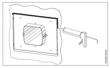
► Use a permanently elastic sealant to seal the joint between the external panel base plate and the wall.
