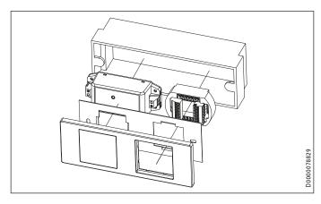
The control unit, the power supply unit and the programming unit are installed together in a double flush box.
