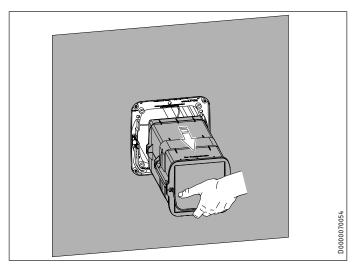
► Use the bracket to pull the fan unit out of the wall mount casing.
