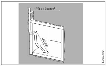
► Secure the wooden edging in the aperture. Use PUR foam, for example.
