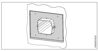
▶ On the outside of the building, push the external cover base plate over the wall mount casing protruding from the wall.
