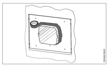
► Affix the permeable film as a vapour barrier to the outside over the joint between the wall mount casing and the external cover base plate.
