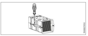
► Screw in the screws on the long sides of the fan unit.
