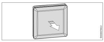
▶ If the internal panel is not open, carefully pull the internal panel cover slightly back from the base plate.
