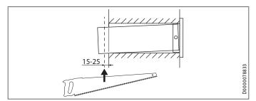
► Shorten the wall mount casing so that it protrudes over the external panel base plate by the length illustrated.
