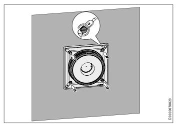
Use the knurled screws included in the standard delivery to secure the internal panel base plate to the wall mount casing.
